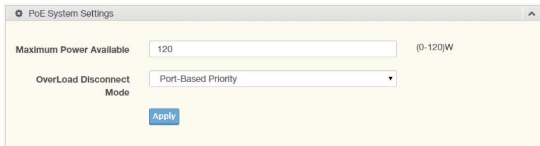
Figure 4.113 Management > Power Over Ethernet > PoE System Settings
