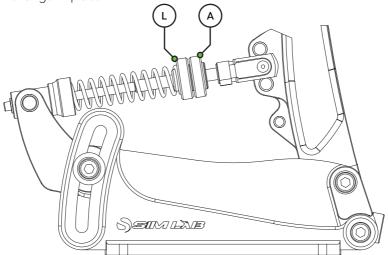
The same principle applies to the maximum travel of the pedal. On the bottom of the pedal arm you will find two blue knobs as well. The inner one is the locking knob (L), the outer one is the adjustment knob (A). Turning the adjustment knob clockwise results in less travel, turning the adjustment knob anti-clockwise results in more travel. By default, the pedal has been setup to provide a middle of the road range of travel but you are free to experiment.
