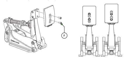
As mentioned, it is also possible to change the angle of the pedal face. Begin by loosening the top (T) (countersunk) bolts, but do not remove them. Temporarily remove the bottom (B) bolts and now the bracket can rotate freely. The bracket comes with a preset slot for different angles you can choose from. Choose your angle and fix it in place using the two bottom bolts (B). When happy, tighten the upper two (T) bolts again as well.
