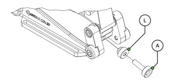
Adjusting spring force isn't only possible by using the adjustment knobs. Using the lower of the three adjustment points on the pedal arm gives you a slightly softer (S) pedal pressure for example. The higher of the three a slightly firmer (F).
