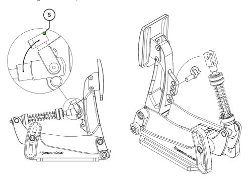
Release any tension from the spring by loosening any adjustment knob(s) before trying to remove the spring bolt.
