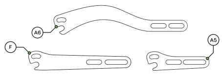
If arms (F) fitted out of the box need to be swapped, first rotate the lever (L) upwards and loosen the nut (N). Now you can disconnect the complete shifter body along with the arms and swap them with your preferred arms (A5/6).
