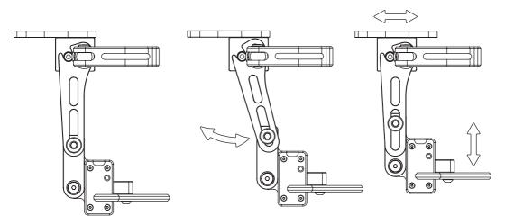
Most adjustments can be made loosening the bolts which hold the arms and rotating the locking lever upwards. Be sure to tighten bolts securely and double check after the first use if they are still tight. Here is how we achieved our setup to work with a deep dish wheel.
