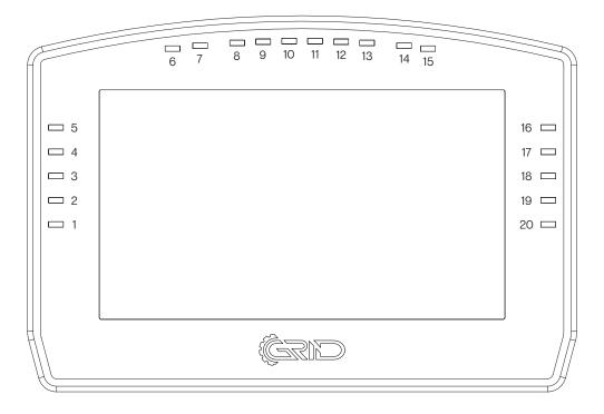
There should be enough info in the sample profile to be able to adjust to your liking. Just keep in mind, you mostly need two values. The number of the LED where you want an effect to start, and the amount of LEDs to use for said effect (in a clockwise direction).
