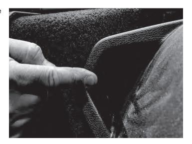
Pop the rear seatbelt cover panel up and pry subwoofer enclosure off the rear quarter panel
