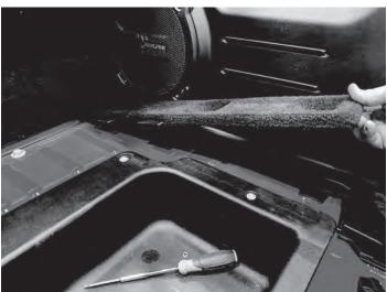
\*For Wrangler 4XE lift up the panel behind rear seat and remove\*
