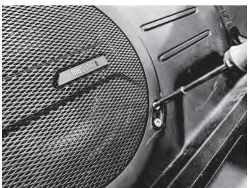
• Place the subwoofer enclosure into the vehicle
