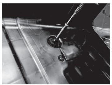
Remove the eight 5mm allen screws from the perimeter of the subwoofer
