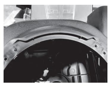
• Install provided wiring harness and grommet into the enclosure
