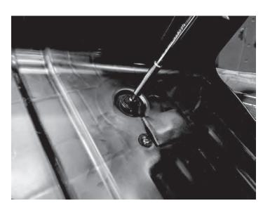
Install the new MB Quart emblem onto the grill, attach the grill and trim ring reusing the eight 5mm allen screws
