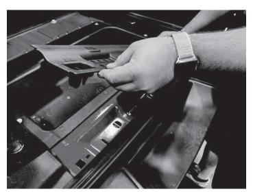
Remove three tie down hooks with T30 Torx Driver and remove side floor
