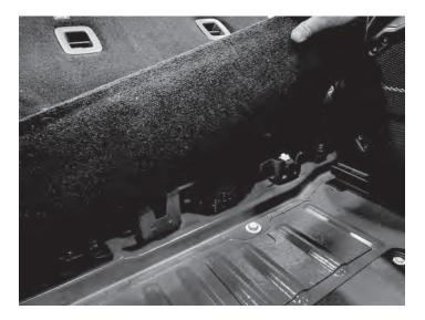
Install floor side panel and three tie down hooks with T30 Torx screws
