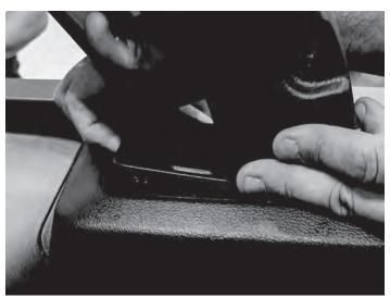
• Reinstall T20 Torx screw to the front of the enclosure
