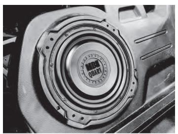
• Install the OEM T20 Torx screw to the rear of the enclosure
