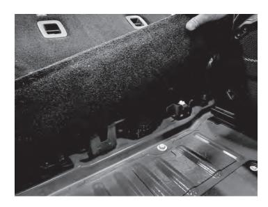
• Remove T20 Torx screw from the front side of the subwoofer panel
