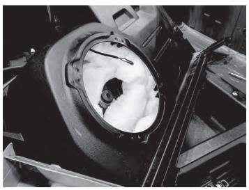
Cut and remove eight plastic tabs on enclosure using a utility knife
