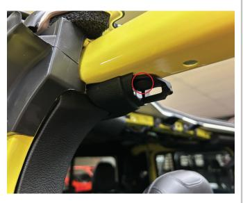
• Unclip the two panels on the b-pillar sill panel.
