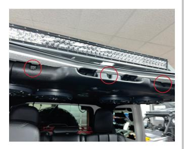
Install the passenger side ROPs panel by carefully sliding into place and then clipping. After, secure with two T25 Torx.
