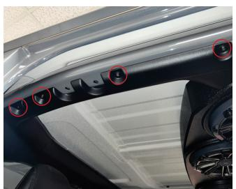
Carefully install the passenger side front ROPs panel by sliding into place then snapping the clips into the final position. Install two T25 Torx screws.
