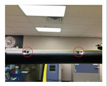
Install two T25 Torx screws on passenger side front ROPs panel.
