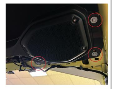
Install the MB Quart Soundbar using the bolts from the previous step.
