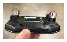
Carefully unclip the middle ROPs cover from the OEM soundbar and remove from the vehicle
