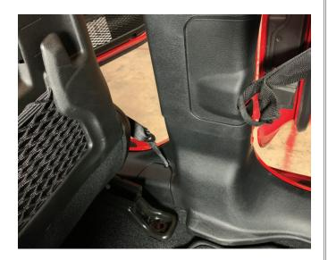
Install passenger side corner panel by clipping back into the vehicle.
