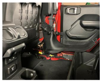
• Disconnect the OEM wiring connector from the OEM soundbar.
