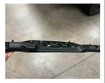
Install dome light wiring connector into the dome light and then clip the dome light into the middle ROPs cover.
