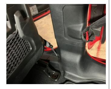
• Unclip the b-pillar sill panel.
