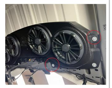
Route the soundbar wiring along the OEM wiring toward the passenger b-pillar sill panel and then down to the floor. Secure wiring with zip ties.
