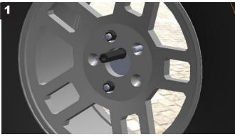
REMOVE 1 LUG NUT AT A TIME ON THE TOP 2 LUGS OF THE SPARE TIRE CARRIER, REPLACING WITH THE Appropriate spacer, thread pitch and length to match your wheel offset and desired look.
