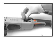
Remove brush side-port screws from both sides of tool using a small Phillips head screwdriver, turning counter-clockwise. Take out the side-port cover. Grasp brass pressure plates and retrieve carbon brushes from tool. Discard appropriately. Install replacement carbon brushes into brush port. Insert the brush side-port cover. Tighten side-port screw using Phillips head screwdriver.
