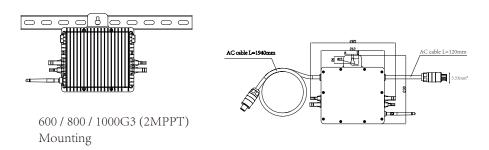
The AC wire on the micro inverter is a TC-ER wire with a wire cross-section area of 3.33 mm<sup>2</sup>.
