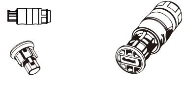
Step 5 - Connect Microinverter to the PV Modules
