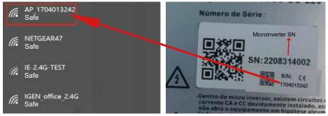
Microinverter SN: 2208314002 Built-in datalogger :1704013242
