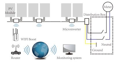
**NOTE**: If the wireless signal in the area where the microinverter is weak is weak, it is necessary to add a wifi signal booster at a suitable place between the router and the microinverter.
