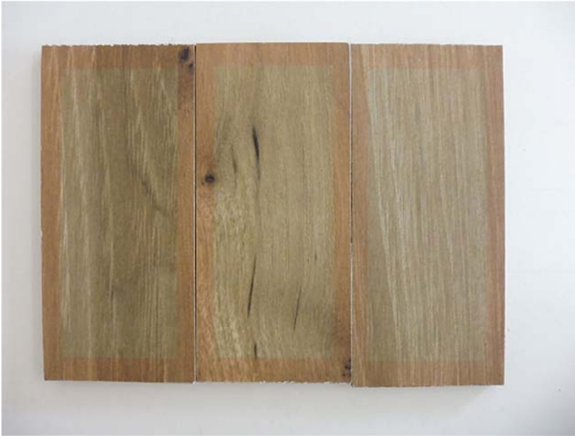
Figure: Test specimens 1 -3 after 3000 hours artificial weathering
