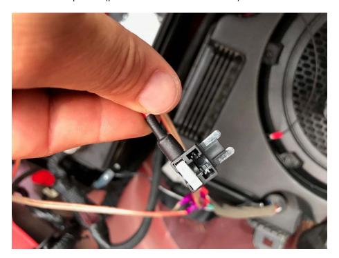
Plug the add-a-circuit into the slot for fuse 37 as shown.
