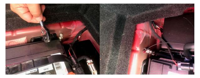
Plug in your Z Automotive device or other compatible OBD2 device and enjoy. A good place to secure it is between the battery strap and the battery.
