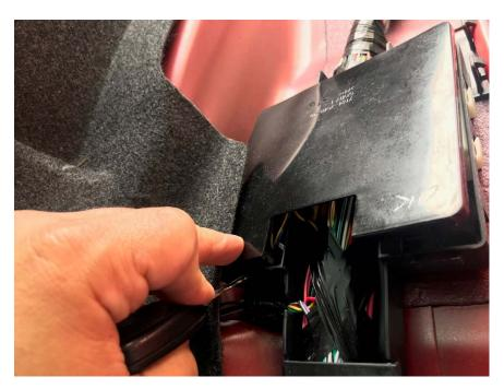
Plug the green plug of the Double Bypass harness into the start connector that has the green plugs. Likewise, plug the white connector into the STAR connector that has white plugs. Any available slot will work.
