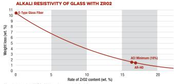
All products tested at 176°F for 200 hours in saturated alkali solution
