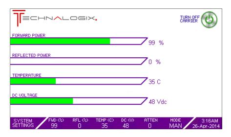
SYSTEM SETTINGS Toggles between Main Screen and Menu Screen. The menu screen has additional settings and monitoring over the Main Screen, and is illustrated in the next section.
