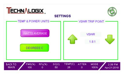
Pressing the DEGREES F button will convert all temperature readings to degrees Fahrenheit from Celsius (and vice versa). Temperature protection trip points are factory set.
