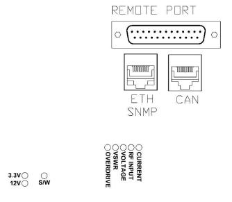
There are (5) fault LEDs, (2) power supply indicator LEDs, and one software LED, as described below.
