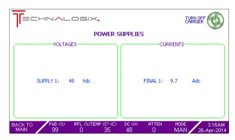
DC supply voltages are nominally 30 or 48Vdc depending on the system. Readings of this voltage in the Power Supplies Screen, and on the summary bar at the bottom of the touchscreen, should not vary more than +/- 2%.
