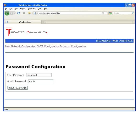
The User account allows access only to the main page. The Admin account allows access to the main and all the configuration pages.
