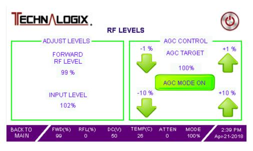
To adjust Forward RF Level (functional only in AGC mode):
