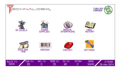
Each of the menu icons on the Menu Screen allow the user to take additional readings or make settings that are not provided from the Main Screen. Any changes to settings will be stored in non-volatile memory with the exception of the date and time which are stored as long as the backup battery remains charged (approximately one week of loss of AC power or power down).
