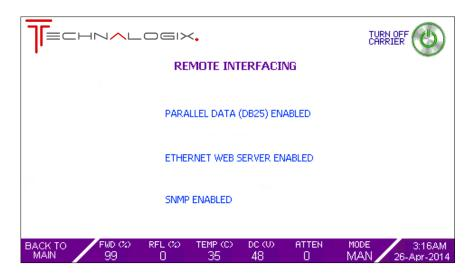
The Remote Port, or parallel data, through the DB25 connector on the back panel of the enclosure extracts the majority of the internal system information and provides it externally for processing and control. The Remote Port is the equivalent of a standalone external remote monitor.
