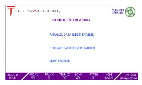
The Remote Port, or parallel data, through the DB25 connector on the back panel of the enclosure extracts the majority of the internal system information and provides it externally for processing and control. The Remote Port is the equivalent of a standalone external remote monitor.
