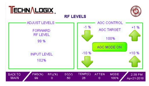
To adjust Forward RF Level (functional only in AGC mode):
