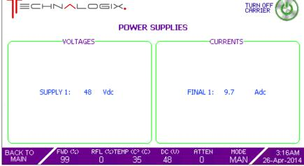
DC supply voltages are nominally 30 or 48Vdc depending on the system. Readings of this voltage in the Power Supplies Screen, and on the summary bar at the bottom of the touchscreen, should not vary more than +/- 2%.
