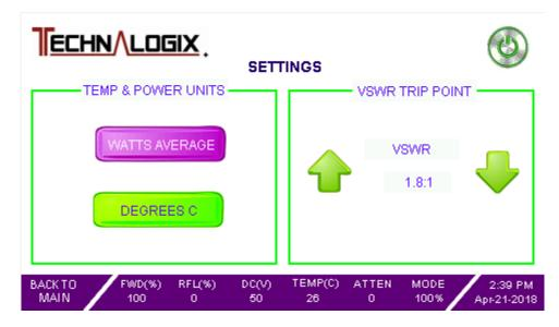
Pressing the DEGREES F button will convert all temperature readings to degrees Fahrenheit from Celsius (and vice versa). Temperature protection trip points are factory set.
