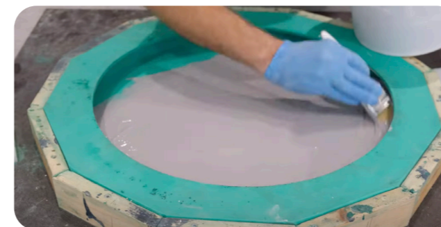
Step Five Brush 1-2mm layer into mould for best results.
