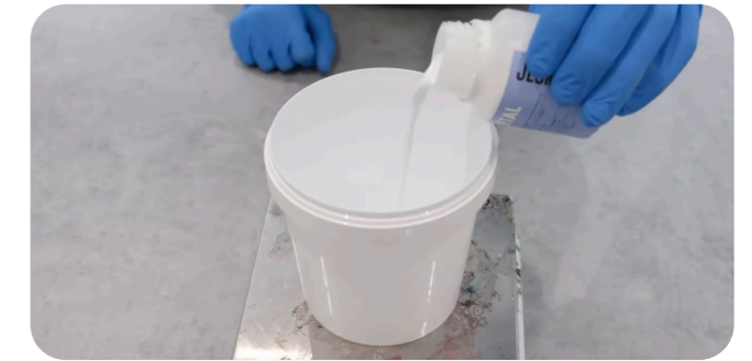
Step Two Weigh out Jesmonite Flex Metal Liquid.
