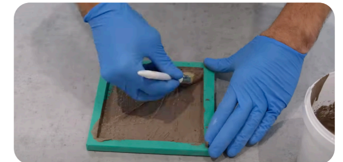
Step Four Brush 1-2mm facing coat into your mould.
