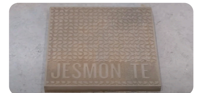
Step Eight Remove from your mould after 24 hours and leave, before polishing to show metal finish.
