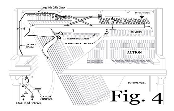
The Quiet Keys unit can be tipped by bending the Mounting Bars so the Muting Rail Felt is positioned close to or touching the Strings when down or in the "on" position.
