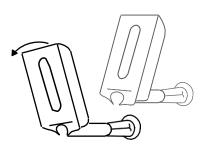
With the On-Off Lever pushed in the Muting Felt should stay above the level of the Hammers allowing for normal function. With the lever pulled out the Muting Felt should drop between the Hammers and Strings of the piano, in close proximity to or touching the strings, muting their volume. Check that metal parts of the Quiet Keys assembly do not touch the piano at any point other than the mounting pins. Check that Pin Collars are securely over pins and that the Wing Nuts are tight.
