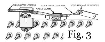
With the Muting Rail "UP", place Cable under Cable Clamp so that its Outer Windings reach half way to the Wire Stop (Fig. 3). Tighten Cable Clamp Wing Nut. The On-Off Control should now move the Muting Rail Up and Down.
