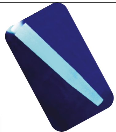
Fig13: Observation of light diffusion through Dentoclic Fiberglass post
