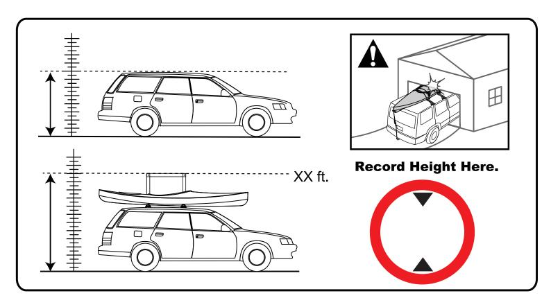
Measure the total height after installation, fill the data in the height limit mark above, tear off the mark and paste it where easily seen inside the car.
