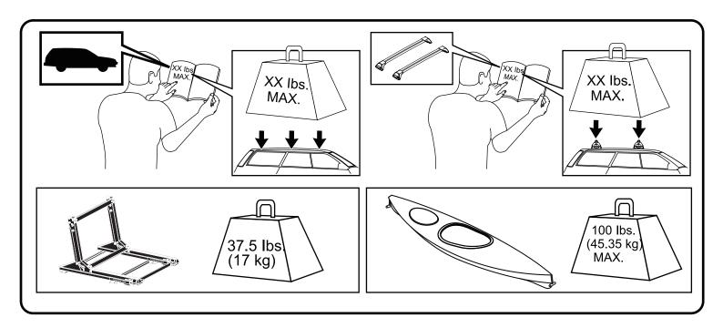
Vehicle must be able to carry 70kg/155lbs total roof load. The minimum load of roof cross bar shall not be less than 65kg/143lbs.Max roof load = load carrier + any fittedcarrier accessories + the weight of the load itself. Refer to thevehicle's owners manual for the maximum load recommended by the manufacturer of the car itself
