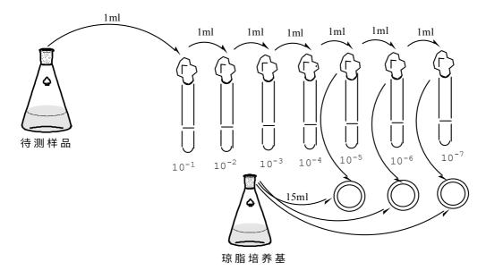
Figure 2-1 Schematic diagram of antimicrobial experiments
