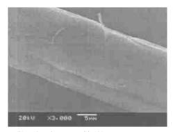
(b) NaOH, the Hemp with 120 □ temperature Figure 3.The hemp fiber scanning electron microscope
