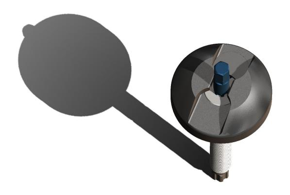
**Step 7**: Torque OneTrax assembly to 55 ft/lb. Filler piece will lock into place.
