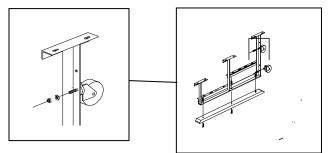
and attached at a later time. Wheels are only attached to the frames at each end of the finished bleacher assembly.
