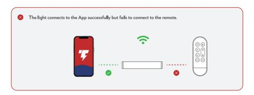
To initiate a remote reset, power on the light and simultaneously press down "ON" and "Brightness -" buttons for five seconds.
