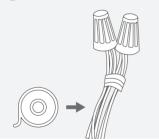
6 Connect all remaining lights to the system then install in place.
