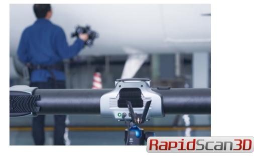
Due to its optical tracking technology, TrackScan-Sharp can precisely measure parts without having to stick reference targets. Its large tracking volume allows users to measure multiple parts at the same time, thus significantly improving operational
