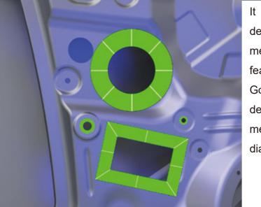
boasts shadow-less-light edge а detection with high-precision gray value measurement. Users can inspect closed features precisely, especially threaded holes. ensured by Good measurements are delivering and repeatable accurate measurement results such as positions and diameters.
