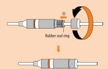
5 Push the rubber seal ring into the waterproof connector and screw the top cover and lock it into position firmly to finish installation
