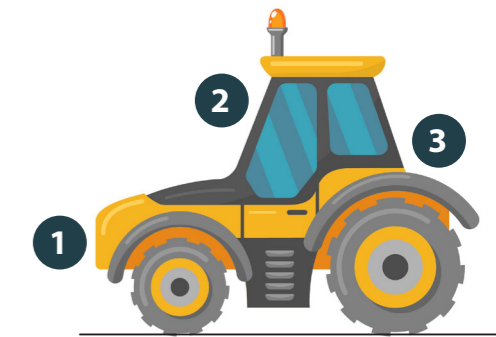
1. Camera 2. Monitor 3. Rear camera
