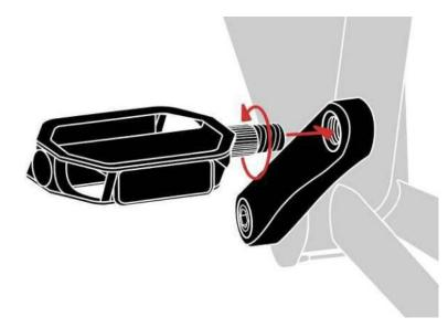
RIGHT pedal: this pedal has no indented lines and is smooth in between the pedal and thread.
