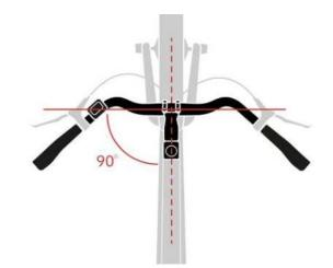
Step 3: Now, using a 4mm allen key, tighten the handlebars and stem, making sure all 4 bolts are centered and tightened properly.
