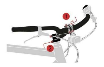
Step 2: Where necessary, loosen the stem bolts and rotate the handlebars in the straight and forward position then align the handlebars so that they are straight and perpendicular to the frame.
