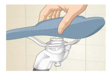
Step 2: Tighten down the clamp bolts to lock the saddle in place.
