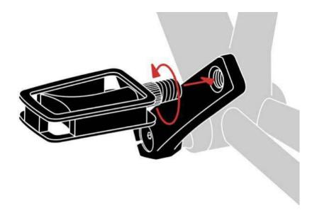
RIGHT pedal: This pedal has no indented lines and is smooth in between the pedal and thread
