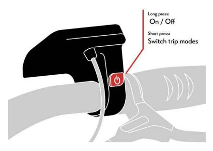
Once on, you can scroll through the 5 levels of motor assist using the + and - buttons on the front of the control module / display. For more in-depth instructions for your screen, please refer to the Bafang manual, found in PDF format on our website.
