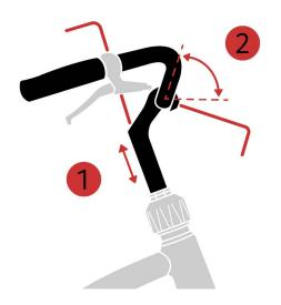
Tip: Should you wish to adjust the angles of you grips, brakes and shifter, you can do so with a simple turn of allen key 3 or 4. However, this should be correctly set already.
