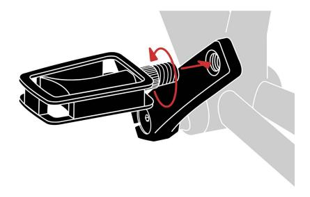
RIGHT pedal: this pedal has no indented lines and is smooth in between the pedal and thread.
