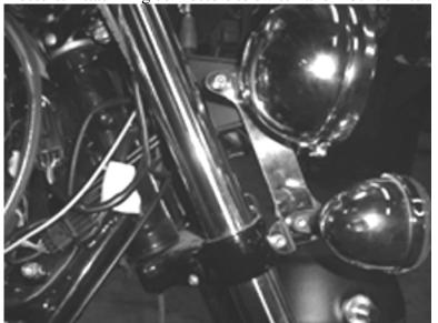
4. Remove the headlight unit and lay it on a towel on the front fender to keep from scratching. Attach each spotlite bracket to the appropriate side. The brackets attach to the turnsignal mounting point and the side screw in the bottom triple clamp. Use the 6x15 mm allen bolts to attach.
