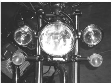
Reinstall headlight. Make final adjustments to positions of spotlites and headlight. Connect to battery
