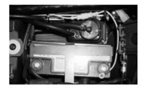
3. Feed front of wire up thru triple clamp and thru dash along handlebar to clutch lever mount. Install the switch bracket on the lower clamp bolt. Determine the proper length of wire needed and cut to appropriate length. Feed remaining wire back thru dash leaving the same amount extending to the switch. Trim two 1" pieces off from the end of the heat shrink tubbing and use the rest to slide down over the exposed wire from the switch to the dash.
