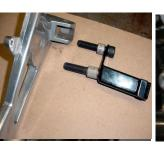
Replace bolts with new bolts and spacers (supplied with our kit) thru the bracket, as shown. Use the spacers between the bracket and the aluminum in the counter-unk holes.
