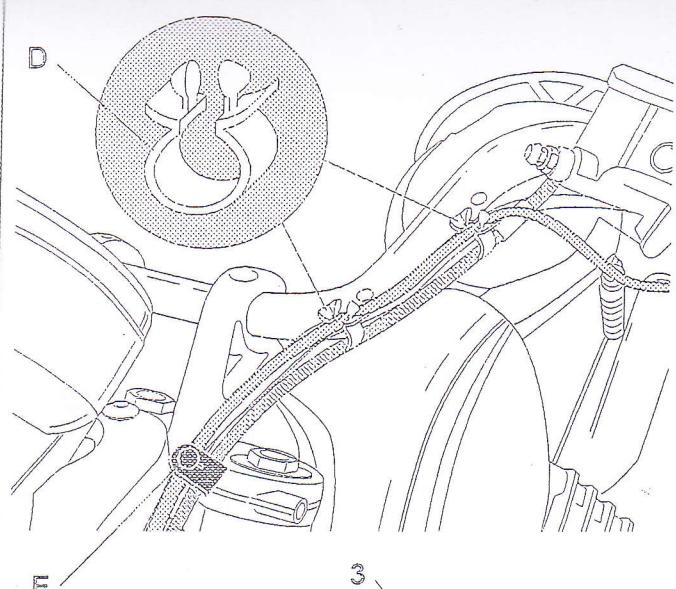
**GB** Remove the two fairleads (D) from the handlebar and replace them with the new fairleads (3) supplied in the kit. Open the rubber fairlead (E).
