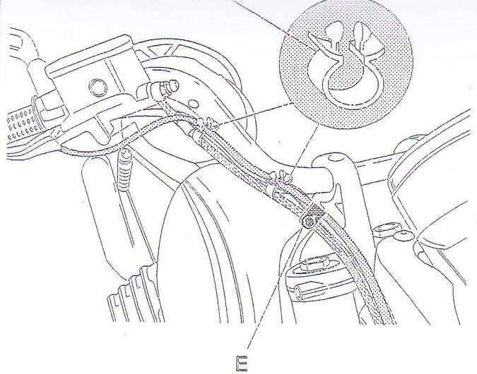
Remove the old fairleads (D) from the handlebar and replace them with the new fairleads (3) supplied in the kit. Open the rubber fairlead (E).
