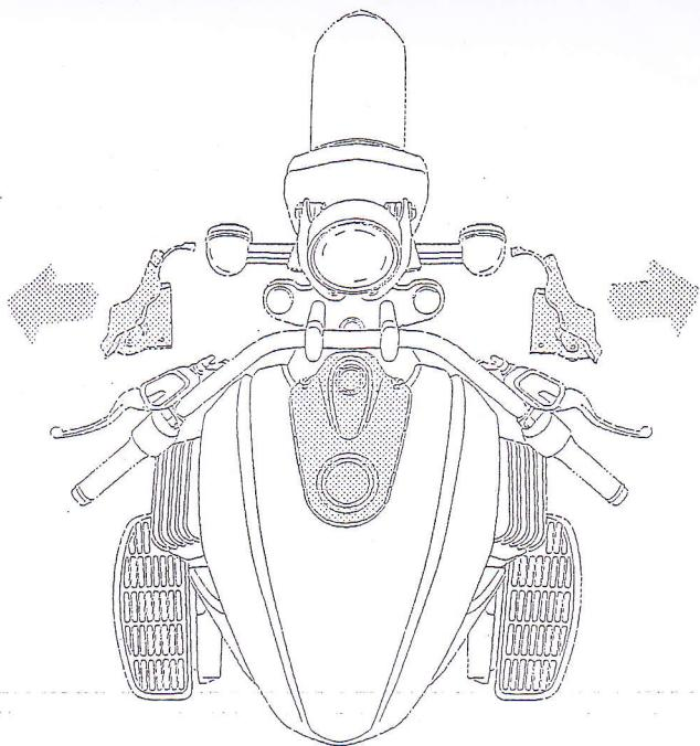
**(E)** Remove the screws and remove the two side panels on the left and right and the cover of the tank.
