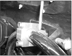
After installing these two sets of clamps in their respective positions proceed to installing the standoffs to the fairing body with the rubber washers and fender washers as per the diagram. (DO NOT TIGHTEN)
