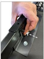
Partially install 2 of the 4 included M10 buttonhead screws. These will be used help connect the base to the shroud.
