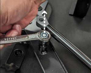
3 Then install the air rod on the stud and replace the washer and nut. Tighten the nut until it contacts the air rod. Do not overtighten. Do this for each side.
