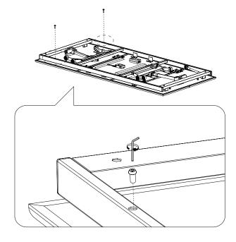
Use at least two (2) people capable of lifting the adjustable base\* into alignment with the gas strut assembly. **Note:** The two partially installed M10 screws should insert into the keyway holes on the gas strut assembly.
