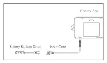
2 Connect the Battery Backup Strap to the (2) Alkaline 9 Volt batteries. Do not mix brand name batteries.
