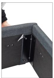
5 Slide all four corner support brackets over the (4) partially installed screws (may need to loosen for install) in each corner. Use the M8 hex key (I) to tighten the screws.
