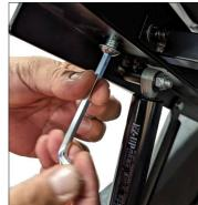
Install the prop rod. The prop rod is a safety device that can be rotated downwards to secure the STOW in an open position. Secure it in place with the provided cotter pin.
