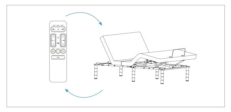
1 Unplug the Power Cord from your power outlet. Wait 1 minute, then plug it back in to your power outlet. Perform Step 2 within 10 seconds, while the control box light is flashing.
