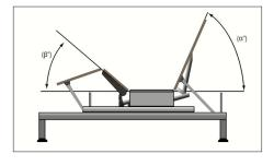
The angle (designated "B" in figure 1) between the flat section and foot section for various configurations of the mattress
