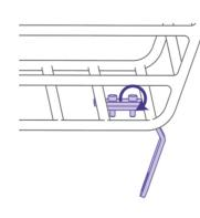
03. Loosen the quick release skewer on the front wheel.
