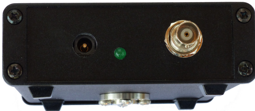
Figure 3.3: End view showing power connector, power indicator LED, and output BNC
