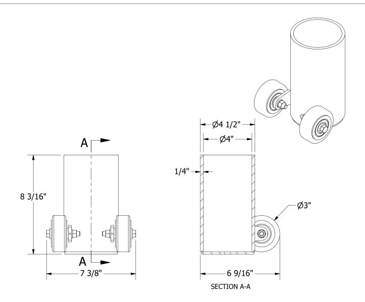
Volleyball pole caddy shall be fabricated of steel tubing with an inside diameter of 4" to allow a 4" diameter volleyball post to be inserted for transport. Two 3" diameter, non-marking wheels shall be attached to the lower section. Welded assembly should be powder coated silver.
