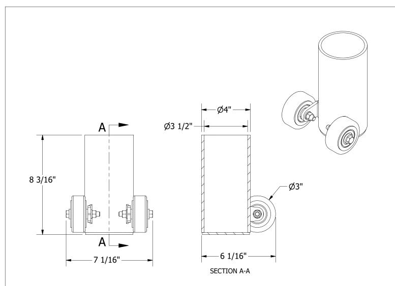
Volleyball pole caddy shall be fabricated of steel tubing with an inside diameter of 3 1/2" to allow a 3 1/2" diameter volleyball post to be inserted for transport. Two 3" diameter, non-marking wheels shall be attached to the lower section. Welded assembly should be powder coated silver.
