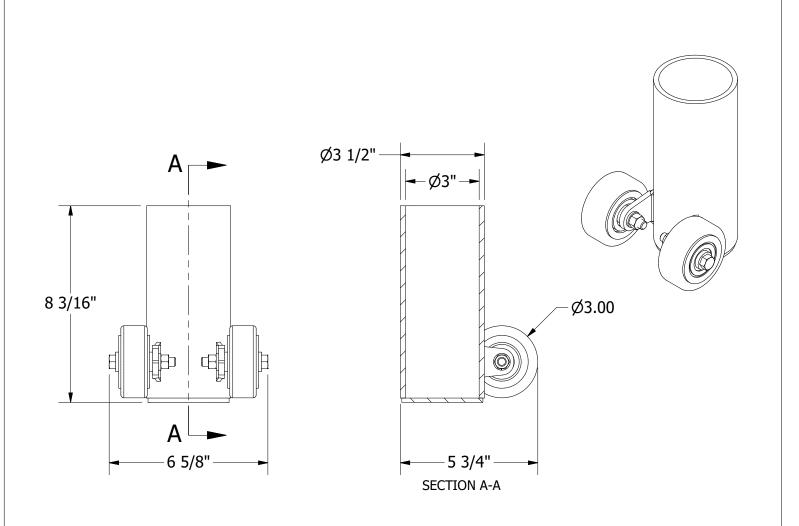
Volleyball pole caddy shall be fabricated of steel tubing with an inside diameter of 3" to allow a 3" diameter volleyball post to be inserted for transport. Two 3" diameter, non-marking wheels shall be attached to the lower section. Welded assembly should be powder coated silver.
