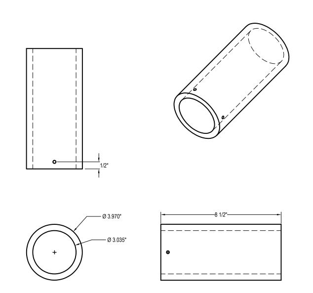
Sleeves are constructed of extruded aluminum tubing with an approximate inside diameter of 3" and outside diameter of 4". Suitable for installing a 3" diameter volleyball post in a 4" diameter socket. The sleeve length is approximate 8 1/2". Two 1/4" diameter threaded holes allow setscrews (provided) to attach the sleeve to either the 3" pole or to the inside diameter of the 4" floor socket or can be used without attachment.
