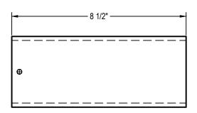
Sleeves are constructed of extruded aluminum tubing with an approximate inside diameter of 3" and outside diameter of 3 1/2". Suitable for installing a 3" diameter volleyball post in a 3 1/2" diameter socket. Sleeve length is approximately 8 1/2". Two 1/4" diameter threaded holes allow setscrews (provided) to attach the sleeve to either the 3" pole or to the inside diameter of the 3 1/2" floor socket or can be used without attachment.
