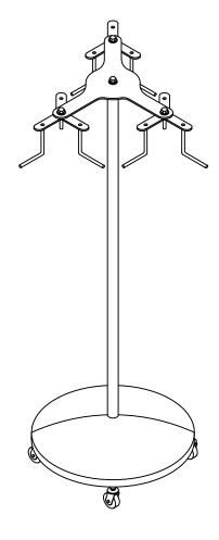
Net storage winder shall be capable of providing tangle free storage of three official volleyball nets in a vertical position. Net winding apparatus and riser pole shall be mounted to a 24" diameter dome shaped base fitted with 3 non marking casters. Entire assembly shall have a gray powder coated finish and weigh approximately 70#.
