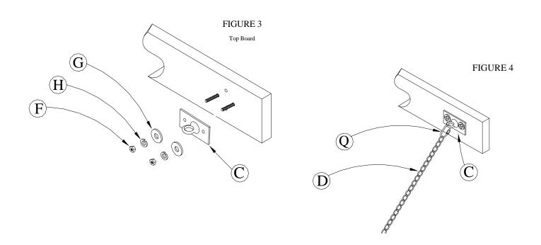
4. Attach a *chain connector* (Q) and a 3/16" proof chain (D) to each *chain eye bracket* (C). (Figure 4)
