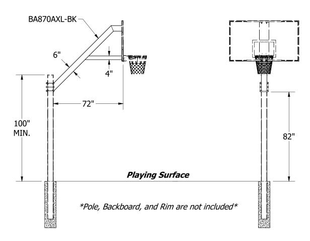
72" setback extension arm shall be substituted for standard 60" extension arm provided with specified system. The substituted extension arm shall be constructed of 6" square, 3/16" wall structured and 4" square, 1/8" wall tubing. Arm shall be mounted to the front of the pole by means of six 5/8" grade 8 bolts. Extension arm shall have a textured black polyester powder coated finish and carries a lifetime functional warranty. Net addition weight shall be approximately 50#.
