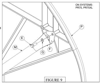
12b. If you are installing a PR74, PR78, PR79, or PR79XL with a BA42UC, BA407U, or BA472PC *Backboard (P)* use 3/8" x 1" Hex Bolts (E), 3/8" Flat Washer (F), and 3/8" Lock Washer (G) to attach the other end of the Backboard Brace (M) to the threaded holes in the rear of the Backboard (P). See Figure 10.
