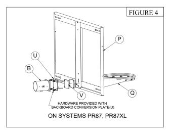
9. Place the assembly from 7a or 7b or 7c above on to the end of the pole. It is easiest to place the assembly onto the end of the pole upside down and then rotate 180° before installing and tensioning the 1/2" Square Head Set Screws (N). Confirm that the Rim (Q) and Backboard (P) are level. Tighten the 1/2" Square Head Set Screws (N) against the Gooseneck Pole (A), then tighten the 1/2" Jam Nuts (O) to lock the 1/2" Square Head Set Screw (N) See Figure 6 and Figure 7.
