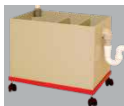
✓ Devices: Sedimentation tanks
