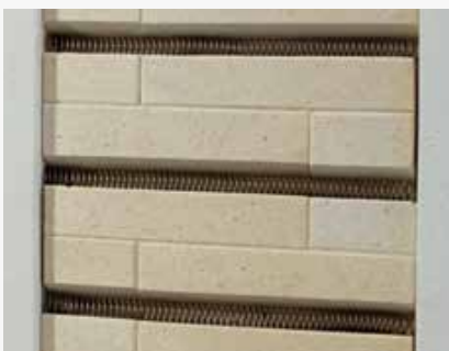
Heating elements in grooved bricks
