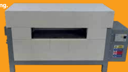
Open high-speed special kiln with removable kiln ceiling.
