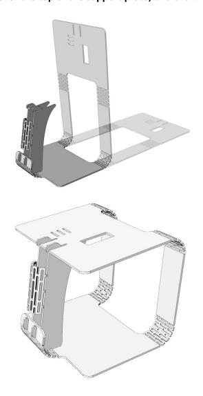
Step 4 - insert one of the phone tabs into one of the three slots on the top of the frame:
