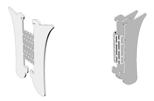
**Step 2 - insert the curved bottom of the support piece into the frame:**
