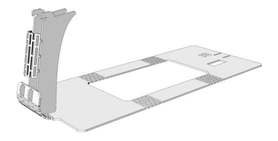
Step 3 – fold the frame over the top of the support piece, and click into place:
